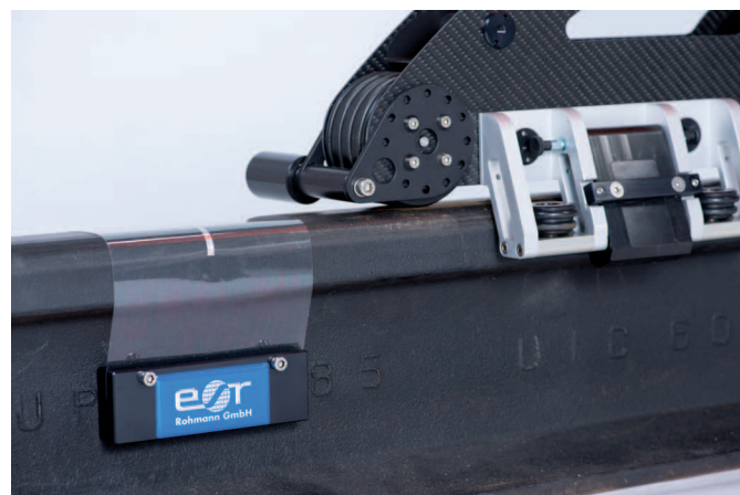
Patented calibration standard with universal magnetic fixture
