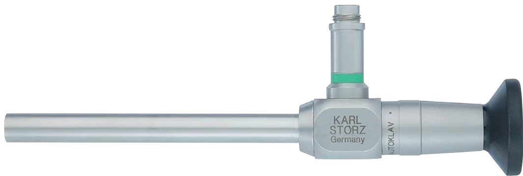
20 9160 20 HOPKINS® Straight Forward Telescope 0° , working distance 25 - 60 cm, diameter 10 mm, length 11 cm, autoclavable, fiber optic light transmission incorporated, color code: green
